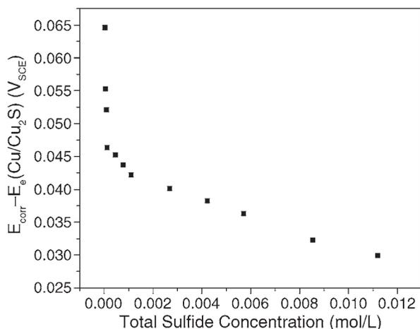
**FIGURE 4.** The difference between the observed  $E_{\text{corr}}$  and the calculated reversible potential ( $E_e$ ) for the Cu/Cu<sub>2</sub>S reaction as a function of total sulfide concentration.
