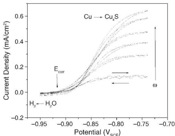
**FIGURE 5.** Voltammetric scans recorded on a rotating disc electrode for  $[S]_T = 10^{-3}$  mol/L at a scan rate of 2 mV/s and various electrode rotation rates (1, 6, 11, 16, 26, 30 Hz). These scans were performed from/to  $-1.35$  V, but only the portion from/to  $-0.96$  V is shown for clarity.
