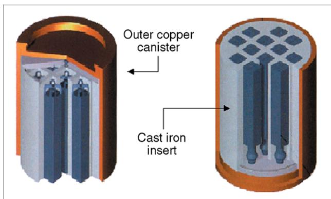
**FIGURE 1.** Schematic of the proposed Scandinavian nuclear waste disposal canister composed of a corrosion-resistant copper outer layer and a carbon-steel inner liner.
