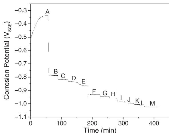
**FIGURE 3.**  $E_{\text{corr}}$  as a function of total sulfide concentration (in mol/L) and time (stagnant solution): (A) 0.00, (B)  $3.32 \times 10^{-5}$ , (C)  $6.62 \times 10^{-5}$ , (D)  $9.90 \times 10^{-5}$ , (E)  $1.32 \times 10^{-4}$ , (F)  $4.59 \times 10^{-4}$ , (G)  $7.84 \times 10^{-4}$ , (H)  $1.11 \times 10^{-3}$ , (I)  $2.69 \times 10^{-3}$ , (J)  $4.23 \times 10^{-3}$ , (K)  $5.71 \times 10^{-3}$ , (L)  $8.55 \times 10^{-3}$ , and (M)  $1.12 \times 10^{-2}$ .
