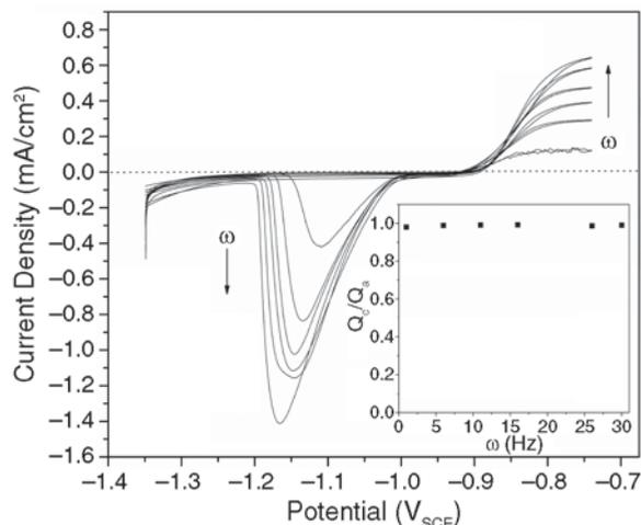
**FIGURE 6.** Voltammetric scans recorded at rotating disc electrodes for  $[S]_T = 10^{-3}$  mol/L (from Figure 5), showing the peaks associated with the cathodic reduction of the copper sulfide film. Inset shows cathodic ( $Q_c$ ) to anodic ( $Q_a$ ) charge ratios obtained by integration of the anodic and cathodic sections of the voltammogram.
