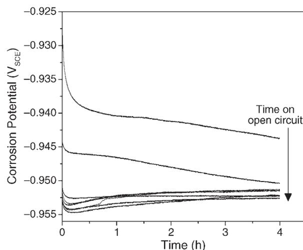
**FIGURE 11.**  $E_{\text{corr}}$  for corrosion in stagnant solution conditions containing  $10^{-3}$  mol/L sulfide.
