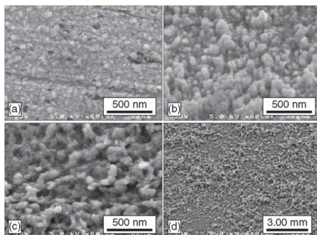
**FIGURE 16.** Scanning electron micrographs of copper sulfide films formed by corrosion in a  $10^{-3}$ -mol/L sulfide solution for a duration of: (a) 1 h, (b) 8 h, and (c,d) 24 h.
