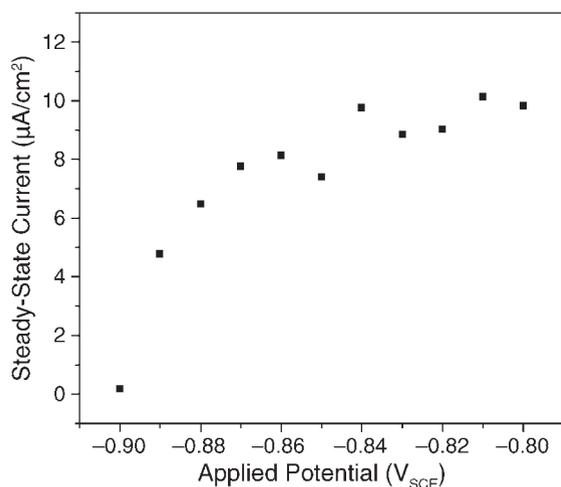
**FIGURE 9.** Plot showing the steady-state current density as a function of applied potential prior to the measurement of the spectra in Figure 8.
