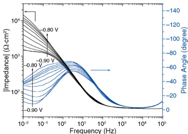
**FIGURE 8.** EIS data (phase angle  $[\theta]$  and absolute impedance  $[Z]$  vs. frequency) as a function of anodic potential,  $[S]_T = 10^{-3}$  mol/L:  $-0.90$  V,  $-0.89$  V,  $-0.88$  V,  $-0.87$  V,  $-0.86$  V,  $-0.85$  V,  $-0.84$  V,  $-0.83$  V,  $-0.82$  V,  $-0.81$  V, and  $-0.80$  V.
