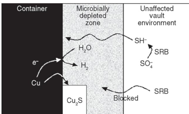
**FIGURE 2.** Schematic illustrating a possible scenario for copper corrosion under anticipated repository conditions.
