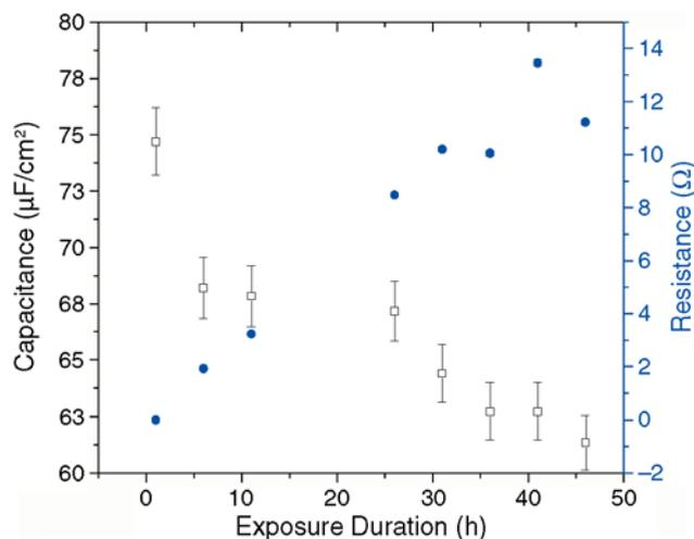
**FIGURE 12.** Total capacitance ( $C_1$ ) and resistance ( $R_1$ ) as a function of exposure duration for a copper electrode in  $10^{-3}$  mol/L sulfide solution. Values were obtained from a fit to the equivalent circuit shown in Figure 10.
