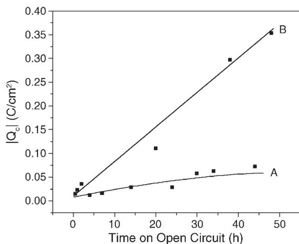
**FIGURE 15.** Plot of cathodic charge ( $Q_C$ ) as function of exposure to a sulfide solution ( $10^{-3}$  mol/L) (obtained by integration of the cathodic peaks in Figures 13 and 14).
