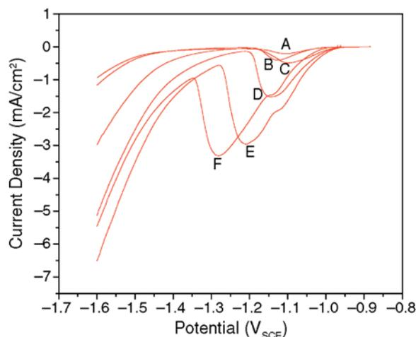
**FIGURE 14.** Cathodic stripping voltammograms recorded after various periods of exposure to a sulfide solution ( $10^{-3}$  mol/L): (A) 0.5 h, (B) 1 h, (C) 4 h, (D) 20 h, (E) 44 h, and (F) 48 h.
