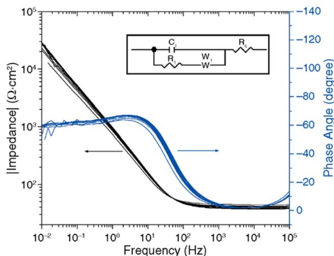
**FIGURE 10.** EIS data recorded during corrosion in a solution containing  $10^{-3}$  mol/L sulfide. This plot includes 10 spectra recorded over the 46-h duration of the experiment. The inset shows the equivalent circuit used to fit the data.
