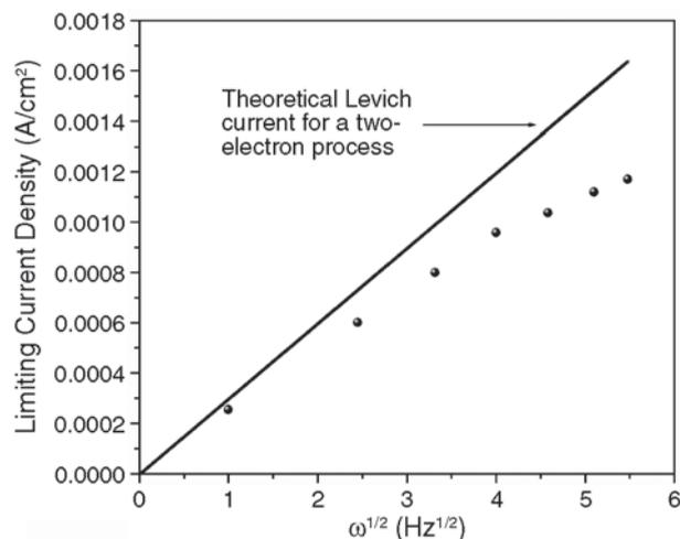
**FIGURE 7.** Limiting anodic currents (from the voltammograms in Figure 5) as a function of the square root of electrode rotation rate ( $\omega$ ), showing that the limiting current approaches the theoretical Levich limiting current as  $\omega \rightarrow 0$ .
