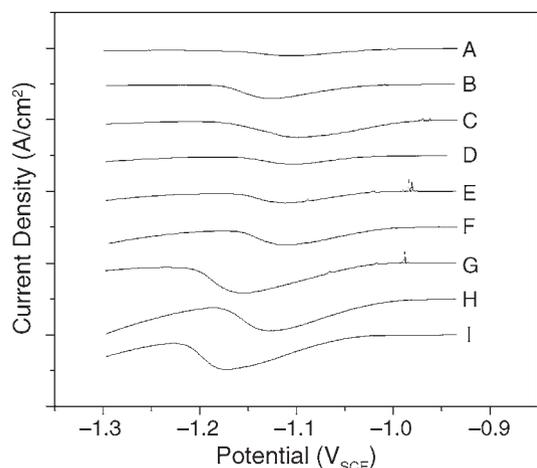
**FIGURE 13.** Cathodic stripping voltammograms recorded after various periods of exposure to a sulfide solution ( $10^{-3}$  mol/L): (A) 0.5 h, (B) 1 h, (C) 2 h, (D) 4 h, (E) 7 h, (F) 14 h, (G) 20 h, (H) 24 h, and (I) 34 h. The current densities have been offset for clarity.
