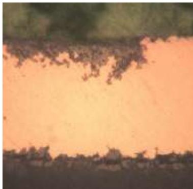
**Figure 2-8.** Cross section through a green-coloured region from one of the copper strips exposed to water in the Pd-sealed flask from Figure 2-7 (Figure 2 of Hultquist et al. 2008/).
