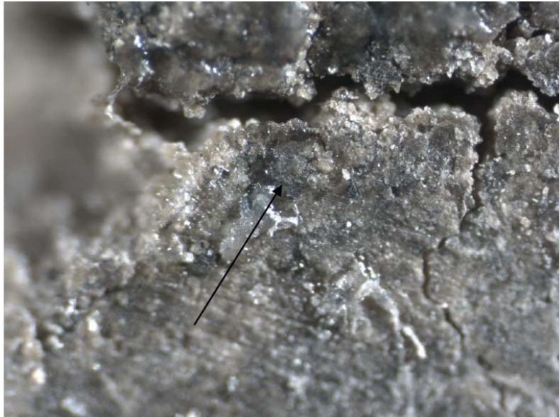
Figure 15: Light microscopy image of the bentonite - Cu tube contact surface (image width appr. 4 cm).
