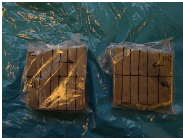
Figure 14: Two slabs marked for cutting 4 radial profiles for the measurement of water content. The profiles are labelled NU (North, upper profile), NL (North, lower profile), SU (South, upper profile), and SL (South, lower profile). The lines marking the cuts for the segments are only approximate
