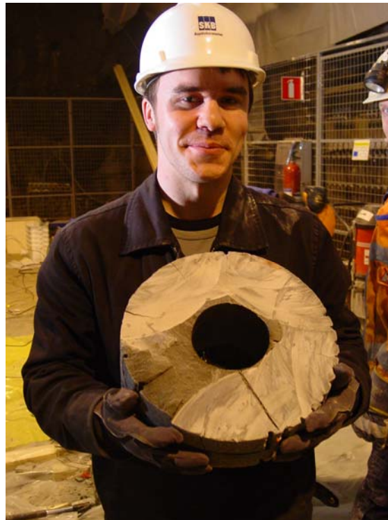
Figure 8: Martin Birgersson from Clay Technology with the successfully removed block 13. The groove marks the top of the block and the North orientation. North is also marked by a red pin placed on the side of the block
