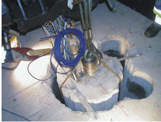
Figure 3: LOT parcel A2 ready to be lifted. The stack of bentonite blocks is completely contained in an outer rind of granite (image from O. Karland, Clay Technology)
