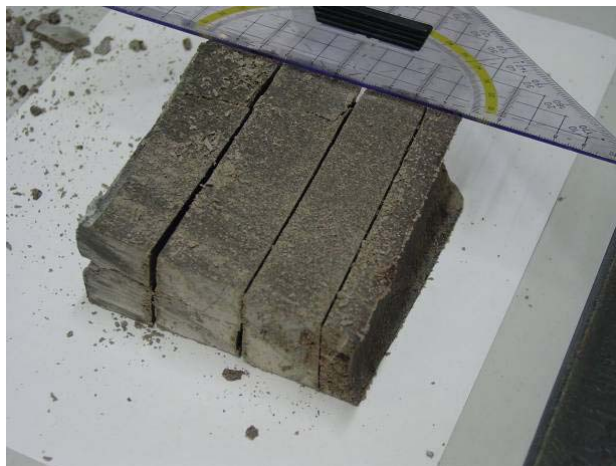
Figure 16: Cut profile from block 13. The heater was in contact along the right side (curved surface), and the contact to granite was along the left side. The lower edge represents the base of block 13
