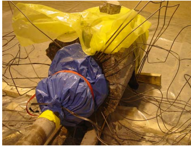
Figure 5: Protection of the bentonite section from drying out between the 1 st and 2 nd day of sampling
