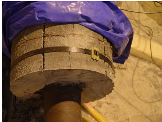
Figure 6: Block 13 secured with a supporting nylon strap, and marked for cutting. The thickness of a block is 10 cm, the outer diameter 30 cm, and the inner diameter 11 cm. The radial width is 9.5 cm
