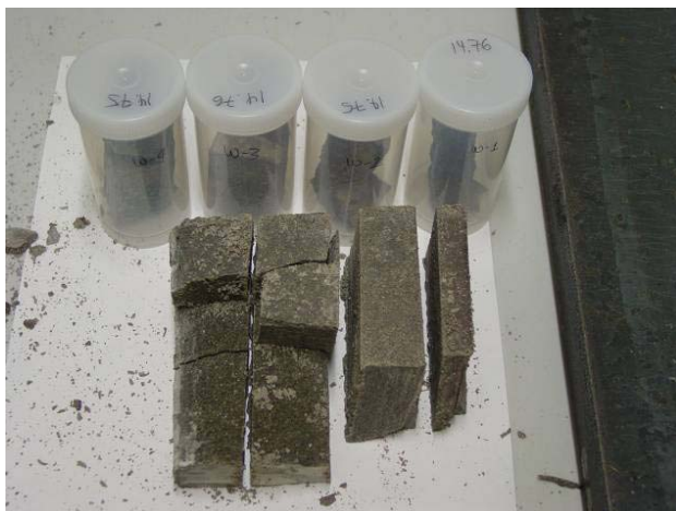
Figure 17: Cut profile from block 13 after subsampling. The larger pieces were processed to perform the CEC, ion selectivity and XRD analyses. Some reference samples were kept sealed and refrigerated (for water content, density)
