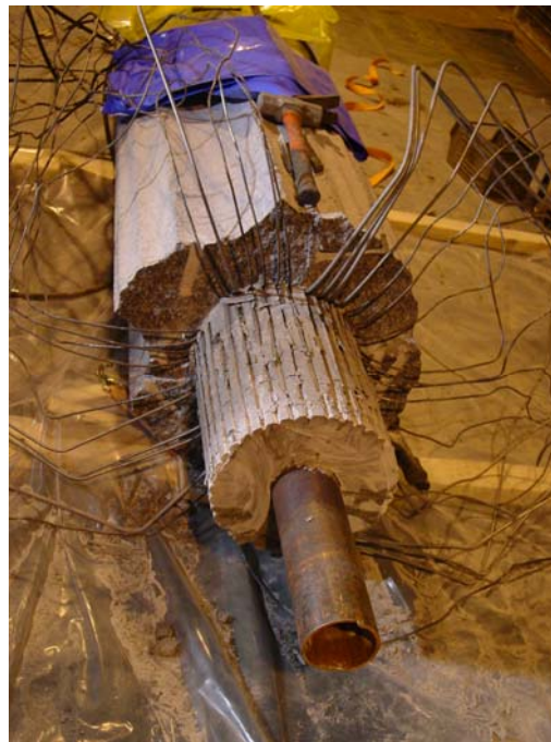
Figure 4: The lower part of the LOT parcel A2. The diameter of the bentonite blocks is 30 cm, stacked on the central copper tube. Sensor wires are located along the outside of the bentonite blocks (peeled back before dissection). The deep end is still contained within a rind of granite
