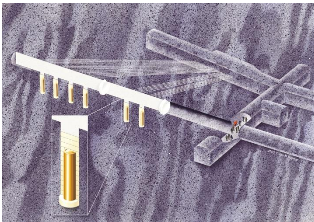
Figure 1. Configuration of the full scale Prototype repository. Initially, a concrete plug sealed the experiment from the rest of the Äspö tunnel and a second concrete plug divided the inner section (four deposition holes) from the outer section (two deposition holes).
