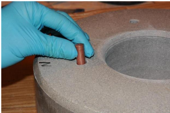
Figure 3. Installation of a copper specimen in one of the bentonite rings in ABM. The hole was sealed with a bentonite plug made from the same material as the ring.
