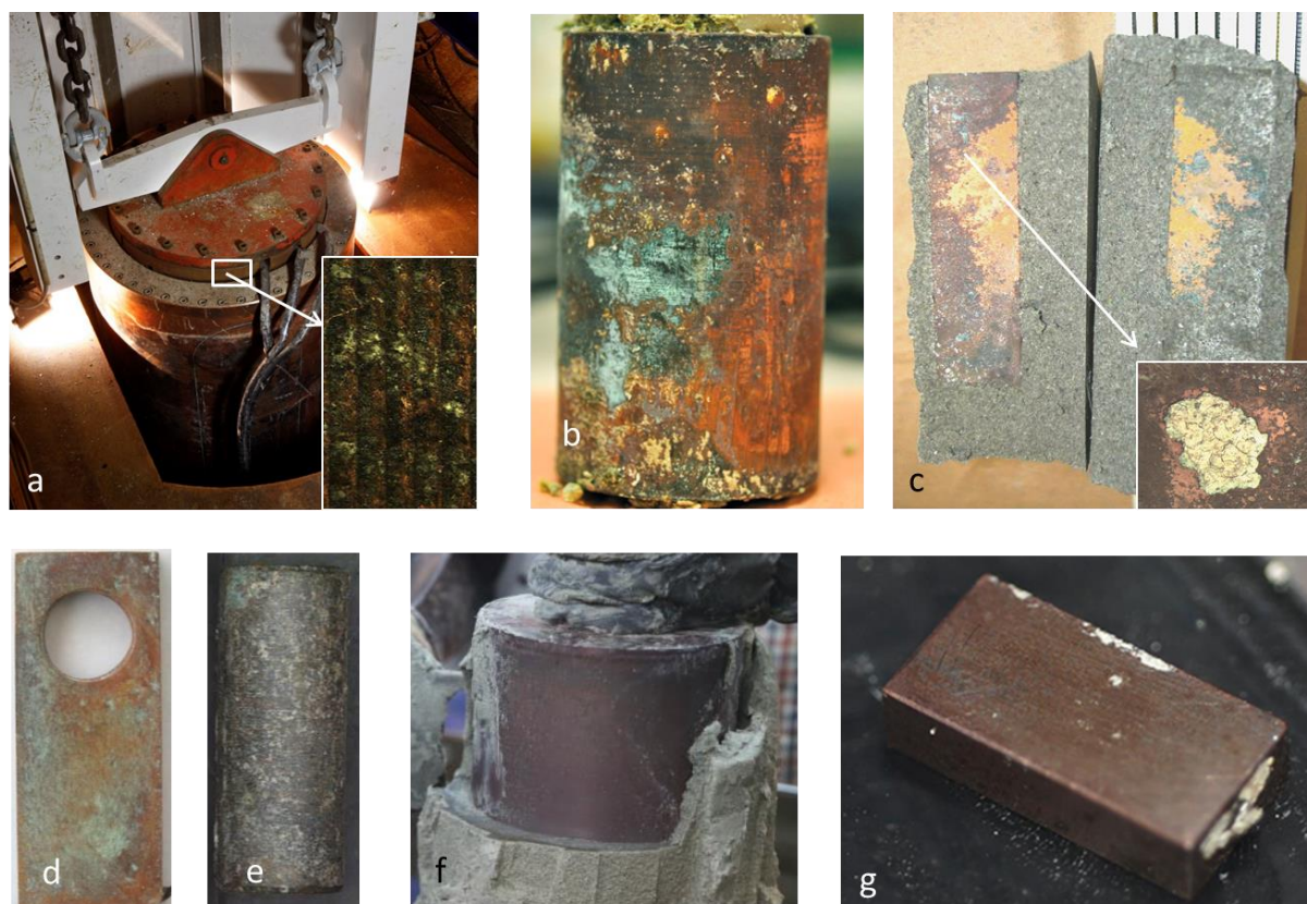
Figure 5. Appearance of copper specimens embedded in bentonite after several years of exposure. a) The canister of PR5 being lifted up from the deposition hole after removal of bentonite clay by drilling. Close up of the corroded surface, both dark brown and blue-green corrosion products are visible. b) The electrode used for electrochemical monitoring in PR5. c) One of the coupons used for mass-loss measurements in LOT/A2. Close up of a blue-green spot. d) Coupon 4A2 from Febex. e) Specimen 13 from ABM 5 f) Bentonite clay being removed from the copper canister of MiniCan 4. g) Copper mass-loss specimen from MiniCan 4 with some bentonite clay still attached to the surface.
