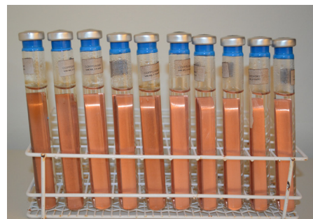
Bild från "Study of H 2 gas emission in sealed compartments containing copper immersed in O 2 -free water", Microbial Analytics Sweden AB
