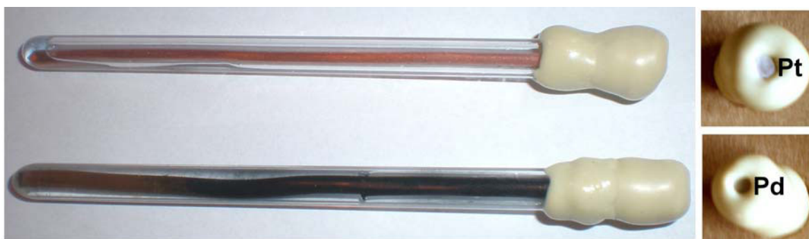
FIGURE 5 –. Appearance of copper after 15 years of exposure in distilled water at room-temperature. Hydrogen is allowed to escape via the palladium membrane from the lower tube but virtually not from the upper tube which has a platinum membrane. The membranes are sealed with UHV-glue (white).
