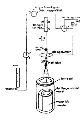
Fig 1: Schematic of reaction vessel and gas sampling system.
