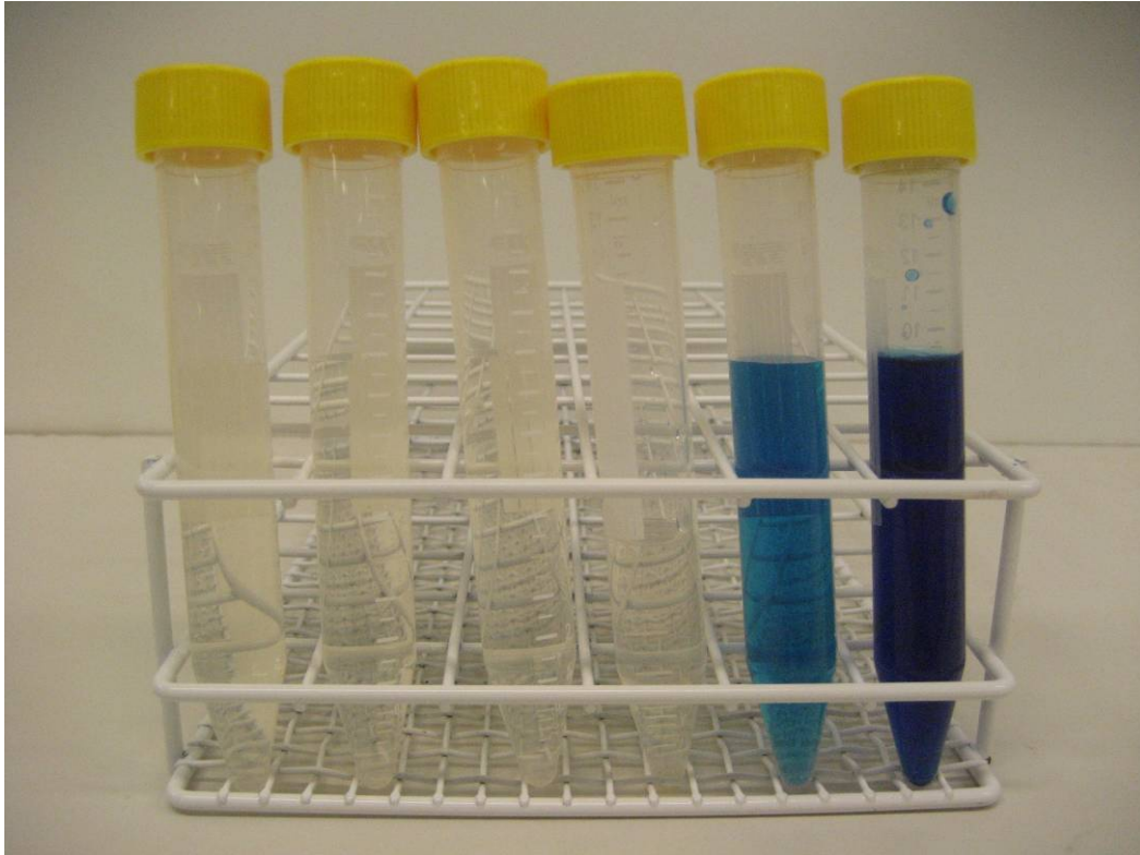
Figure 9-1. Sulphide analysis using the methylene blue method, performed on pore water from a reference and from sampling points KB613, KFA02, KFA03, KFA04, and KFA01. The intensity of the blue indicates how much sulphide is present in the sample; it can be converted to a concentration by measuring the absorbance on a spectrophotometer and subsequently comparing the results with a standard curve.
