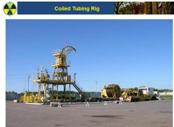
This is the sort of coiled tubing rig needed for emplacing waste packages, retrieving them if necessary, and sealing the hole. It is much smaller than the drill rig.
