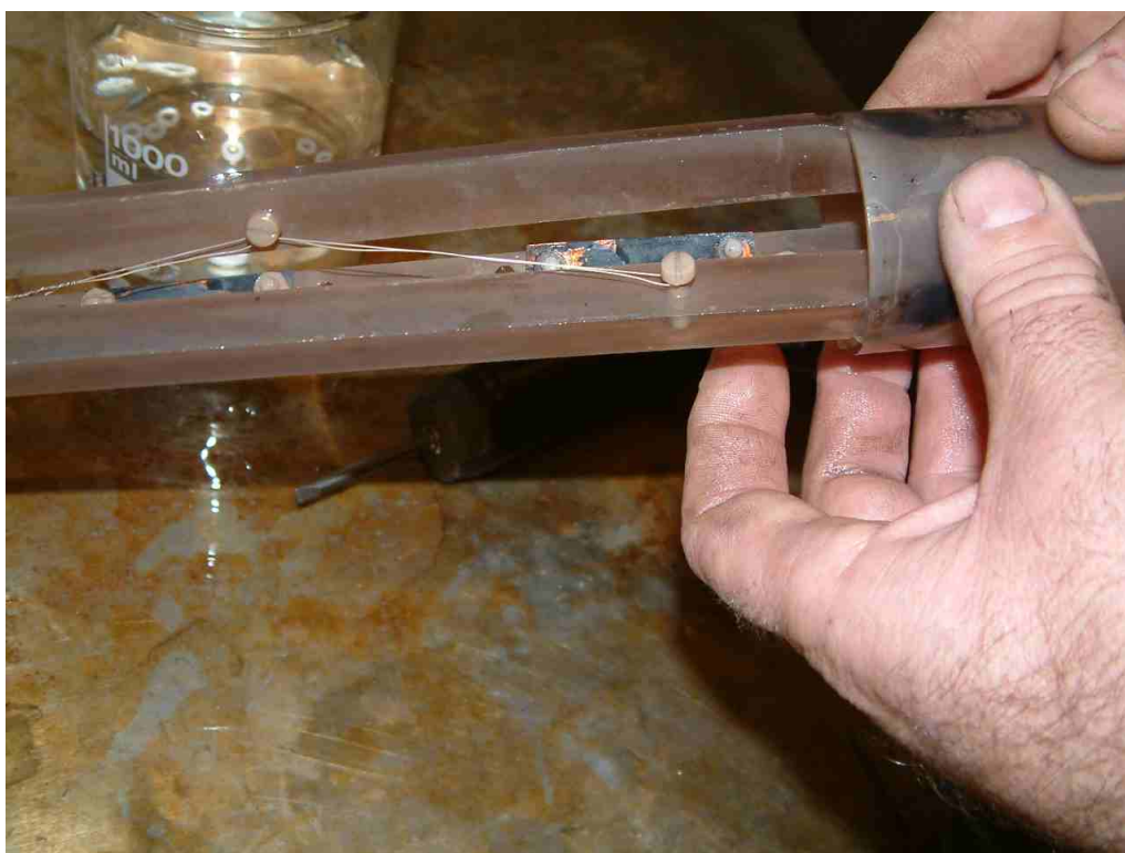
Figure 4. Dismounting the equipment exposed in the sulphide rich water at site SA 1420A.
