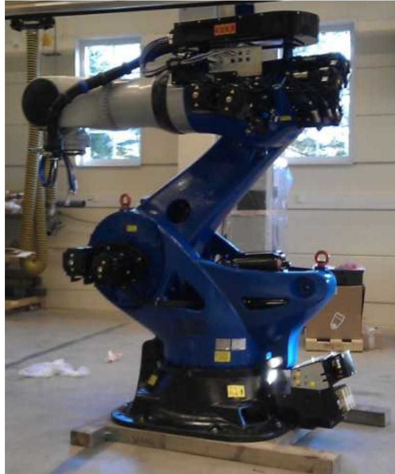
Robot (Backfilling of deposition tunnels)
