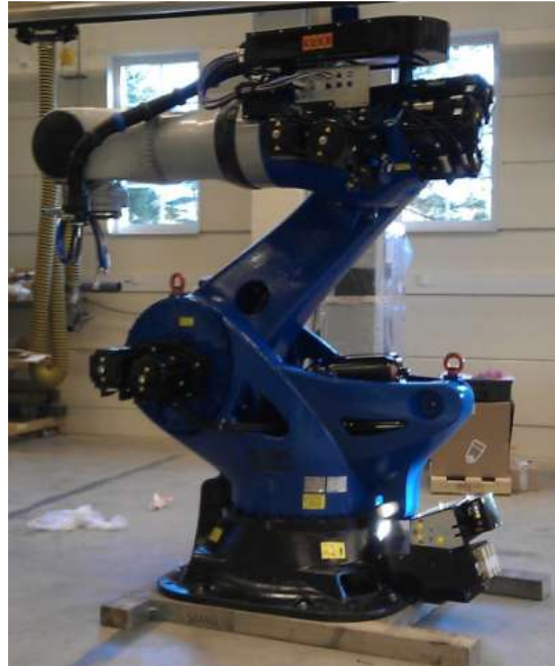
Robot (Backfilling of deposition tunnels)
