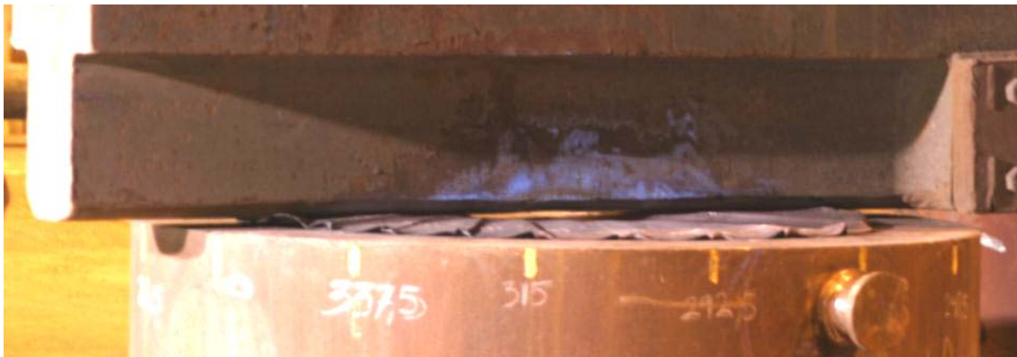
Figure 1-4. Cogging with tools and workpiece shown.
