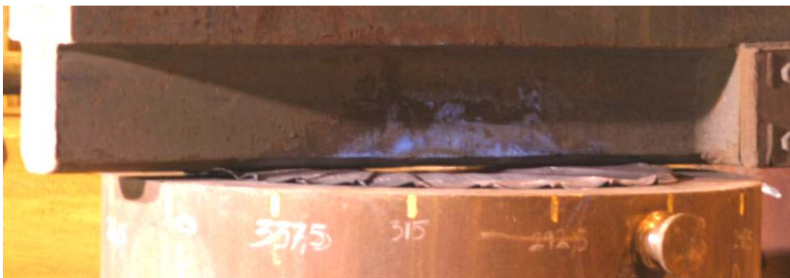
Figure 1-4. Cogging with tools and workpiece shown.
