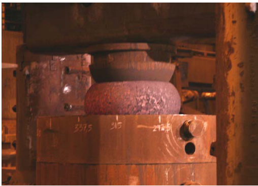
Figure 1-3. The state where the upper tool is pressed 190 mm into the workpiece.
