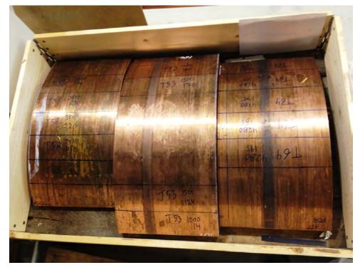
Figure 1. The three different tube pars received for testing. The markings show the different positions for the creep specimen blanks.
