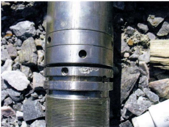
Figure 2-3. Pitting corrosion on the outside of the chemical analysing equipment.
