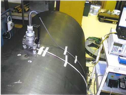
Figure A1:3 The hole drilling rig cemented to the sample.
