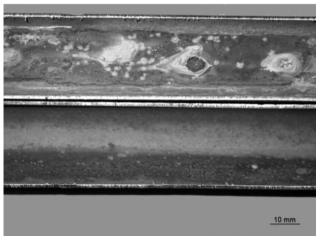
Figure 1. Pitting corrosion on copper pipe
