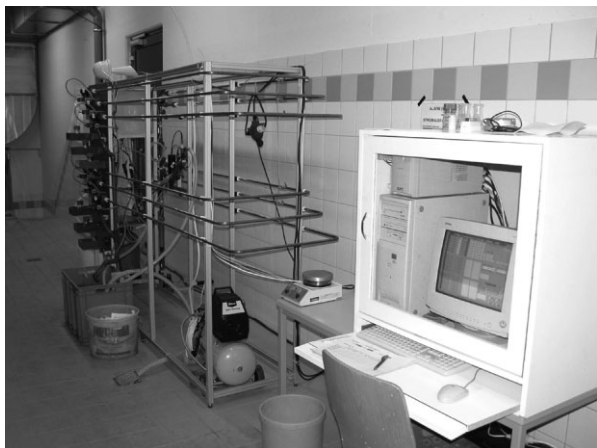
Figure 3. Pilot plant for copper corrosion tests according to DIN 50931-1
