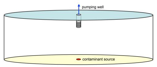
Not to Scale: Model domain has a radius of 10 km and depth of 2 km. Contaminant source has a cross-sectional area of approximately 1  $m^2$ .
