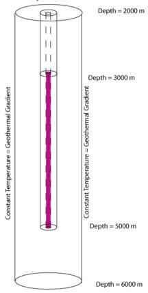
Constant Temperature 160 deg C Constant Hydrostatic Pressure
