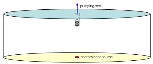
Not to Scale: Model domain has a radius of 10 km and depth of 2 km. Contaminant source has a cross-sectional area of approximately 1 m<sup>2</sup>.
