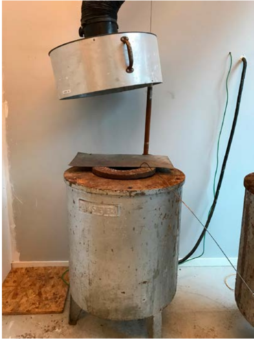
Figure 2-5. The salt bath used for soft annealing of the Bofors creep specimens at 600 °C for 10 minutes.
