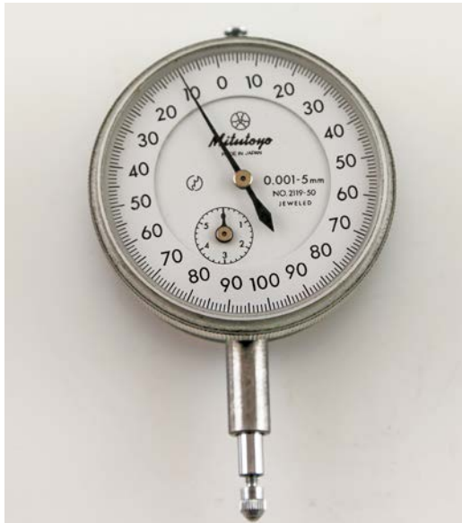
Figure 3-6. The analogue dial indicator with 1 \mu\text{m} in resolution used for measurement of elongation.
