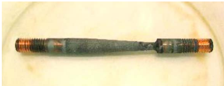
Figure 3.3. Example of SSRT exposed sample, 9 % strain at the thinnest part of the tapered sample (not exposed to final fracture).
