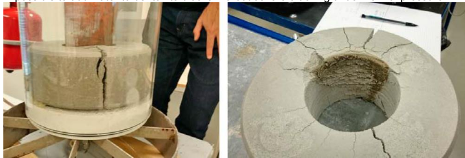
Figure 2.6. From Figure 2-8 in SKB TR-15-09. Left: Test 3 at termination. Right: Bottom side of the bentonite ring showing a condensation “nucleus” and cracks. Severe cracking of the bentonite rings occurred already within 7 days, which was the experiment duration time.
