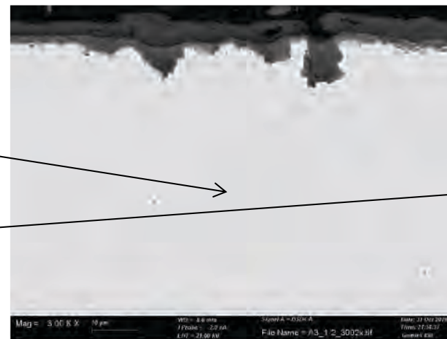
Image of pitting corrosion on the copper tube in the middle of the tube (no detailed results from hottest part of tube)
