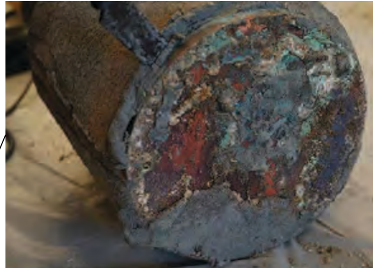
Image of corrosion on the copper bottom plate at 80° C in contact with sand ( no detailed results were in the report, nor of the hottest part of the copper tube )
