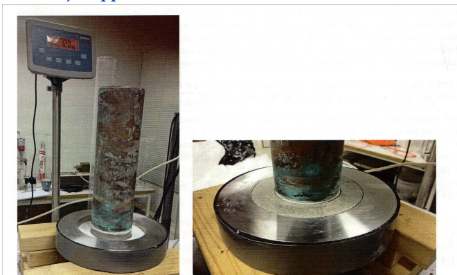
Figure 2-1. Left: copper heater and steel bottom plate. The plastic filter (white) is visible at the bottom of the groove. The outer diameter of this groove is 18.2 cm, and the inner diameter is 10.8 cm. Right: bentonite ring emplaced.
