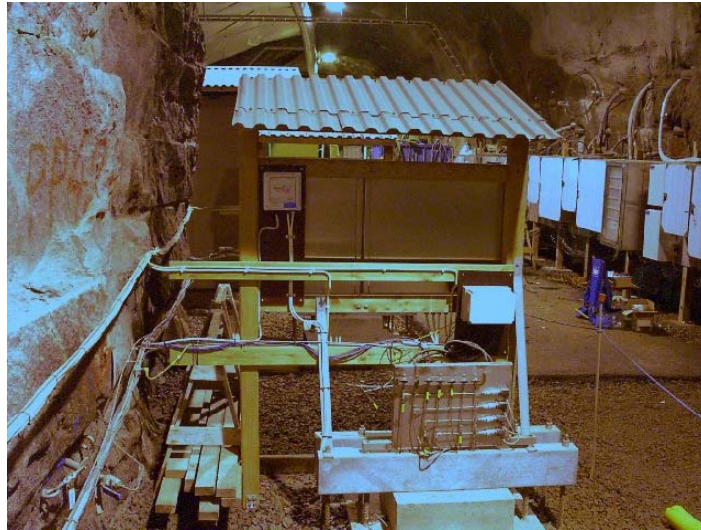
Fig. 4 Top of LOT test parcel A2 with part of the monitoring equipment.
