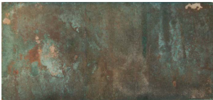
Fig. 7 Appearance of copper coupon S122A after exposure and ultrasonic cleaning in water.
